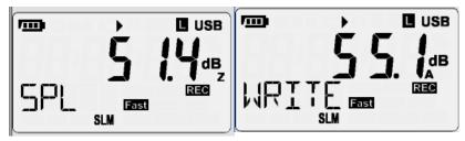
Press the button to enable the auto data record function. The REG symbol will flash on the LCD display. The bottom left of the LCD display will show **WRITE**, at each sample interval to indicate that the data was written to the meter's internal memory.
