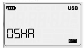
Press the A or button to select a NDM testing regulatory body abbreviation: OSHA, MSHS, DOD, ACGIH, ISO85, ISO90, and USER.
