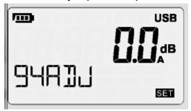
See section on meter calibration before proceeding with this parameter. Press the **SET** button to move to the next parameter or Press enter - to exit set up mode.
