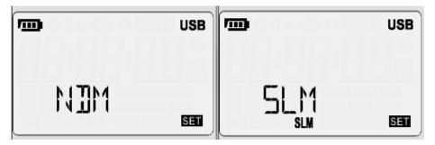
Press the or volume or button to change the test mode between NDM (Noise Dose Meter) and SLM (Sound Level Meter).
