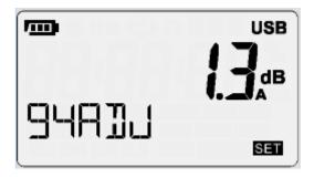
Press the Enter  $\stackrel{\bigodot}{\bigodot}$  key to save the entry and to get back to the measure window. The meter should now read 94.0dB (+/- 0.1dB).
